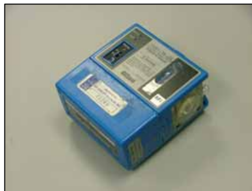
Figure 12: Formaldehyde Sampling Pump
