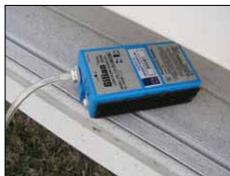
Figure 13: VOC Vacuum Pump
