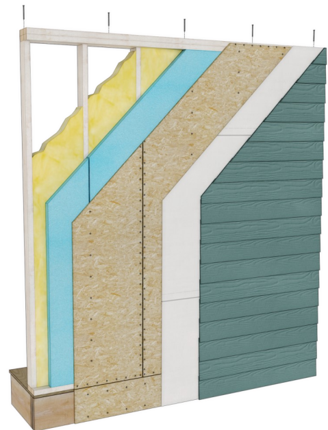
Figure 14. Nails EP&B Walls require modified nailing patterns.
