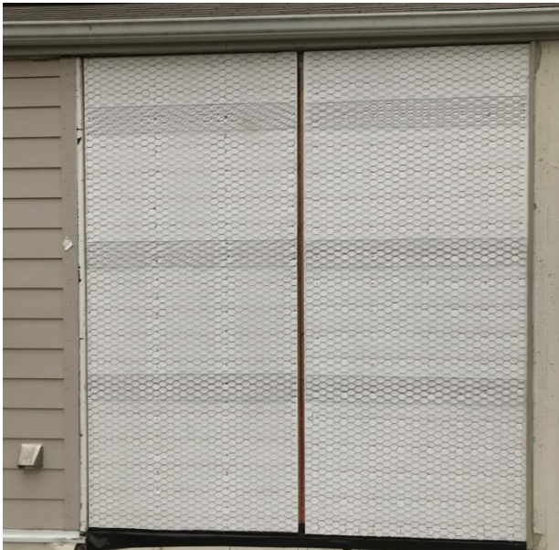
Figure 24. Two 4-ft. x 9-ft. Outdoor Specimens - Construction
