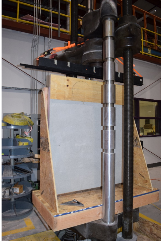
Figure 35. UTM with 4-ft x 4-ft Wall Specimen
