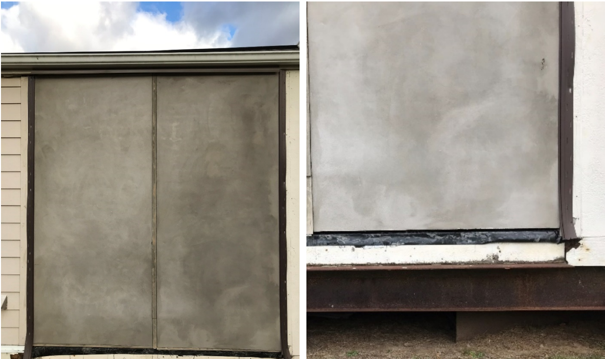
Figure 27 Completed Outdoor Specimens; Right Side of R-H Specimen Shows the Effect of Surface Water
