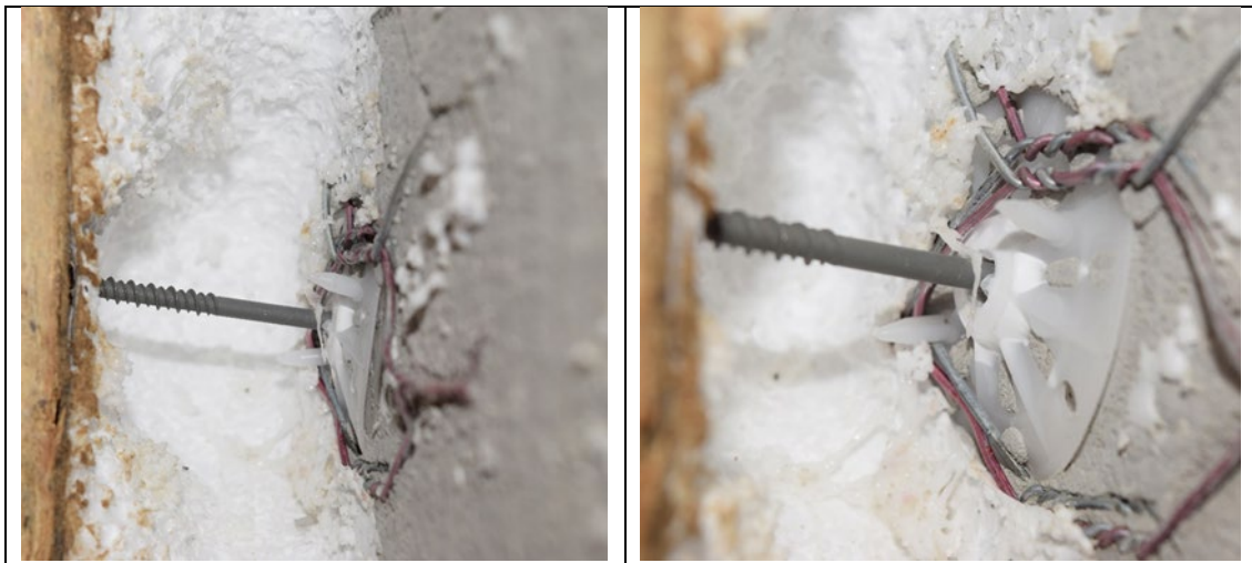
Figure 15. Screws with Plastic Washers – Failure Mode
