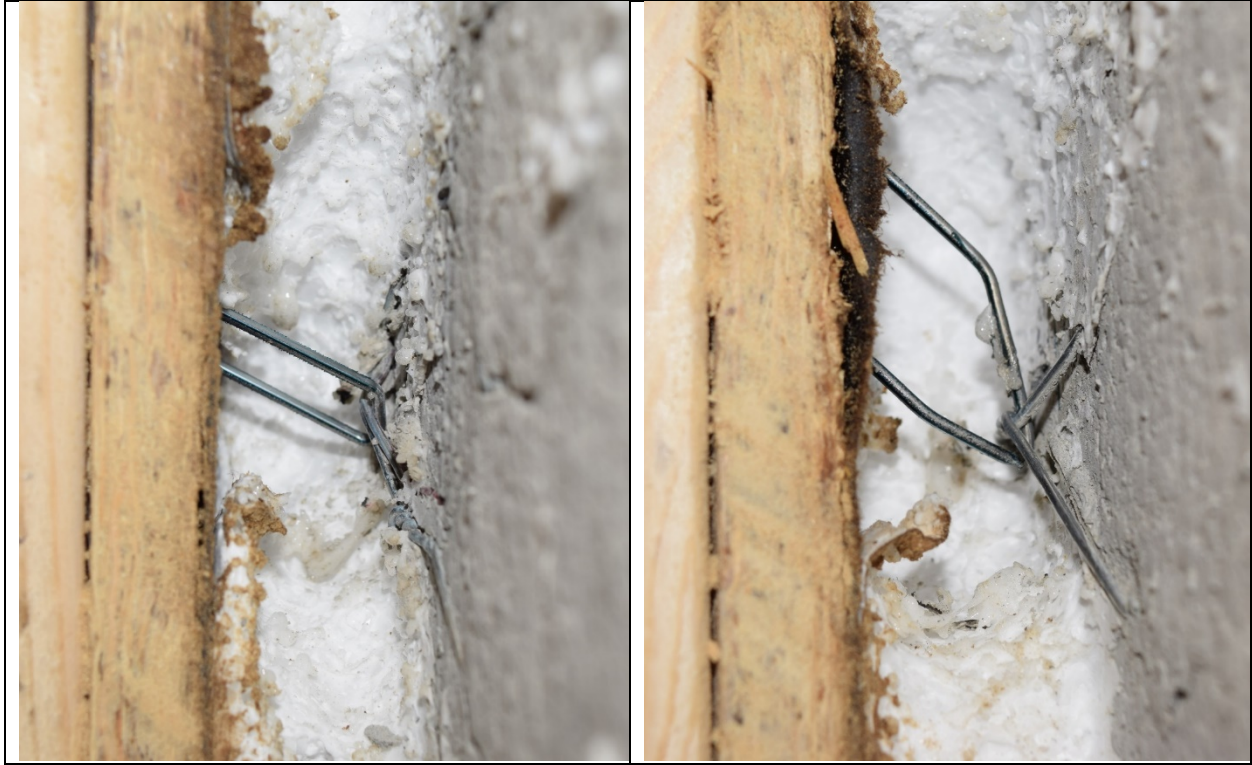
Figure 19. Staples with Different Crown Widths – Failure Modes
