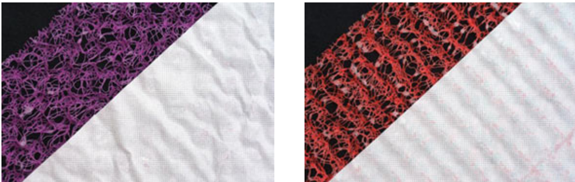
Figure 41. Woven Plastic Filament Drainage Mats Used in Specimen Construction – L: 1/4-in.; R: 3/8-in.
