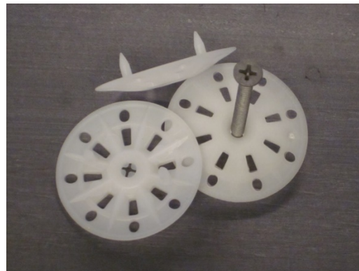
Figure 39. Metal and Plastic Washers Used in Specimen Construction
