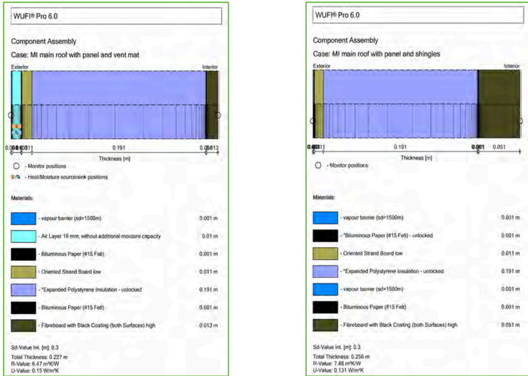
Figure 15. Main roof component assembly for the Michigan house
