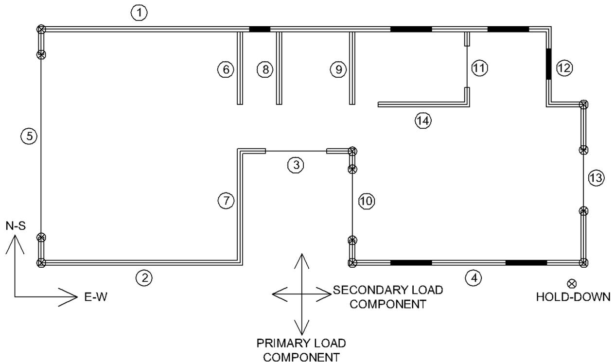
Figure 4 - Shear wall layout of NEESWood Project test house
