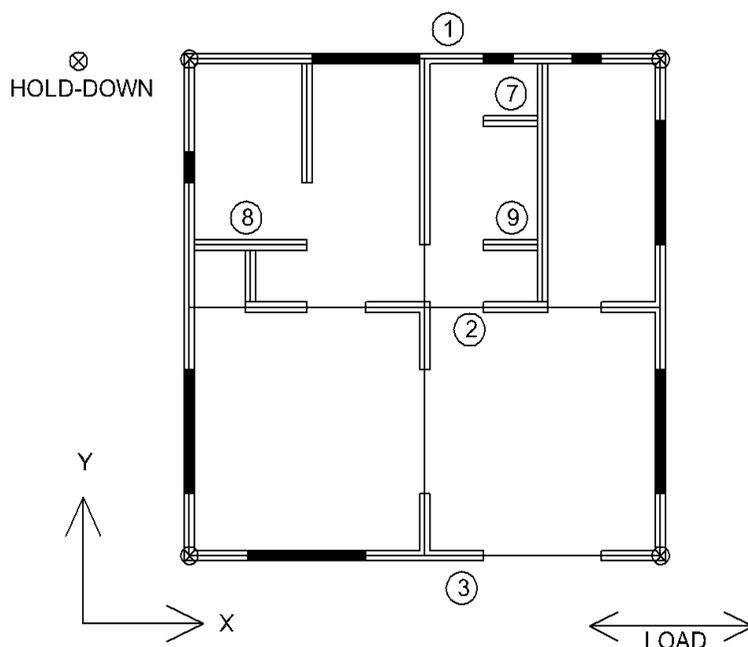
Figure 6 - Wall layout of test house
