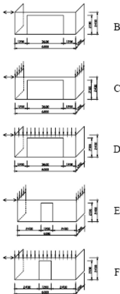
Figure 7 - Configurations of shear walls tested during Forintek/Tongji project
