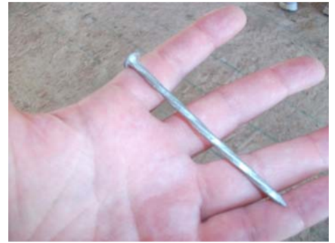
Use a 3-1/2-in. spiral or ring shank nail where direct engagement to framing is desired for added security.
