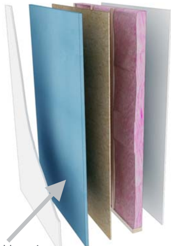
Typical location of rigid foam: exterior to WSP
