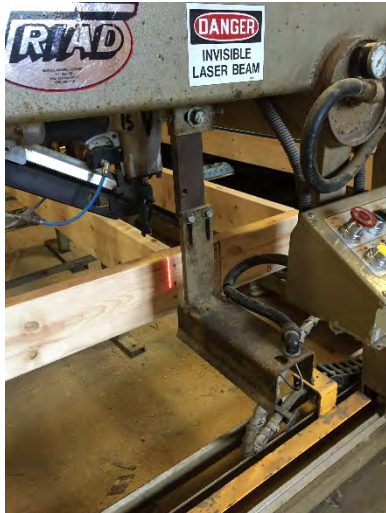
Figure 49. Laser sight bridge nailer
