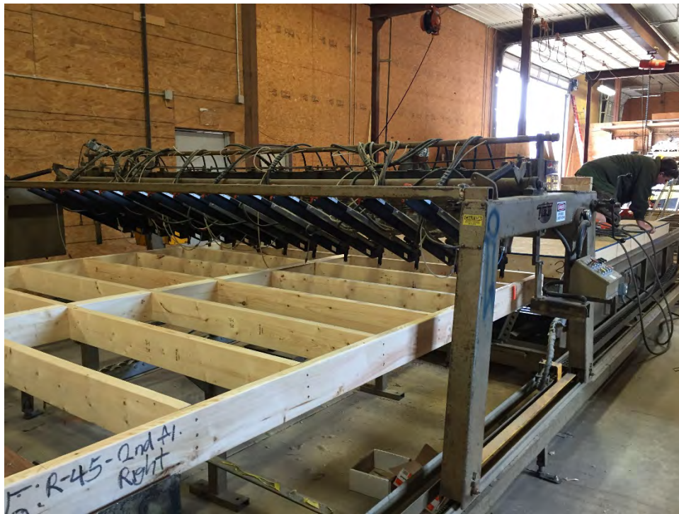
Figure 48. Bridge nailer, Zeeland Truss & Components
