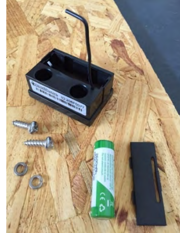
Figure 11. Omnisense T/RH%/MC% sensor
