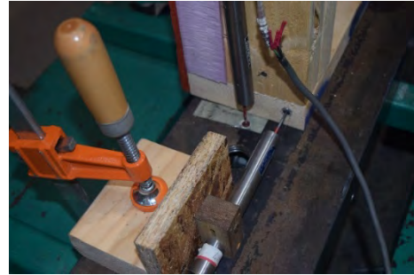
String potentiometer for measuring uplift, displacement
