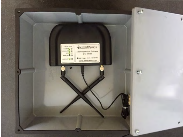
Figure 10. Omnisense Gateway data acquisition unit
