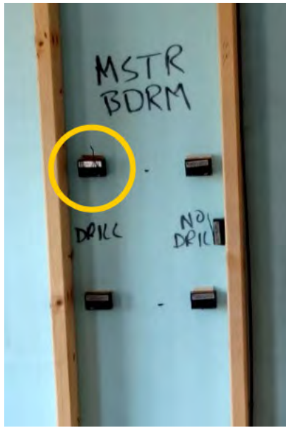
Figure 69. Detail of outlier OSB sensor, House 2
