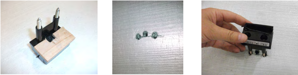
Figure 71. A spacer ensures proper embedment depth into the OSB.
