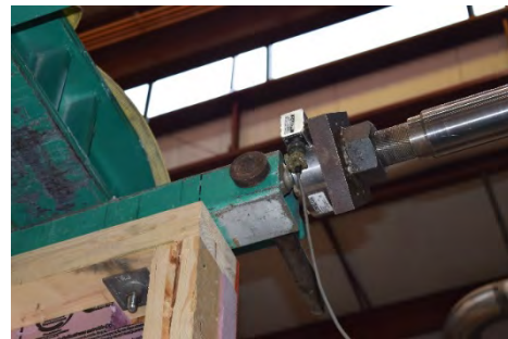
Boundary conditions: loading beam, plate anchors
