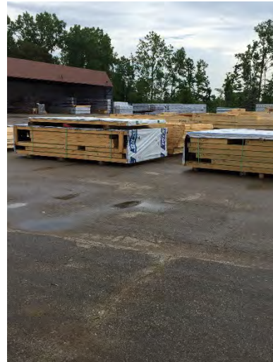
Figure 50. Wall panel bundles ready for shipment
