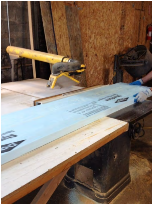
Figure 57. Cutting XPS on a table saw
