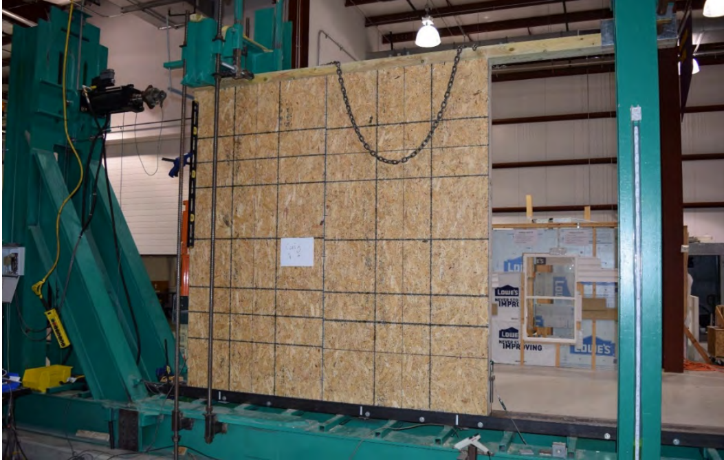
Figure 44. A 2x6 standard reference wall in testing apparatus prepared for ASTM 72 test
