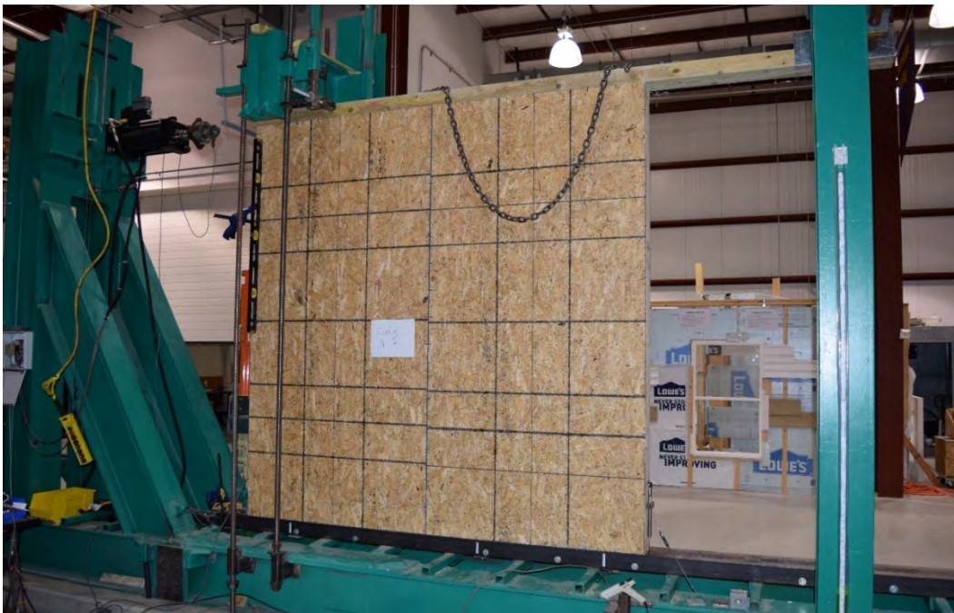
Figure 4. A 2x6 standard reference wall in testing apparatus prepared for an ASTM 72 test
