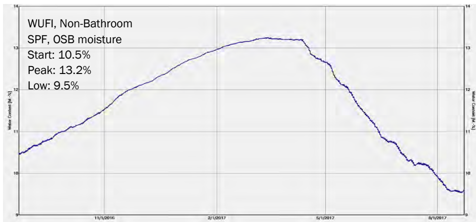
Figure 38. Comparing actual OSB MC to WUFI simulation, Grand Rapids test houses, spruce-pine-fur
