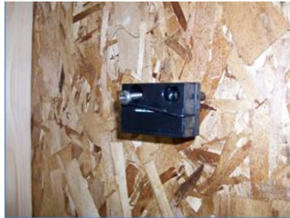
Figure 8. Screws used to Install Moisture Sensors
