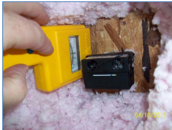
Figure 55. Moisture Meter Reading Correlated with Sensor
