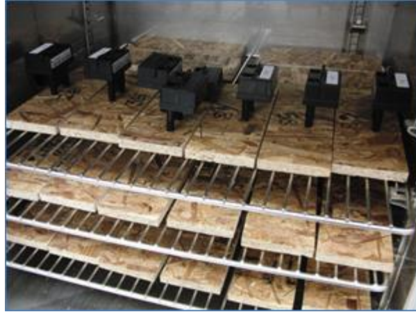
Figure 9. Sensors in the Environmental Chamber for Calibration
