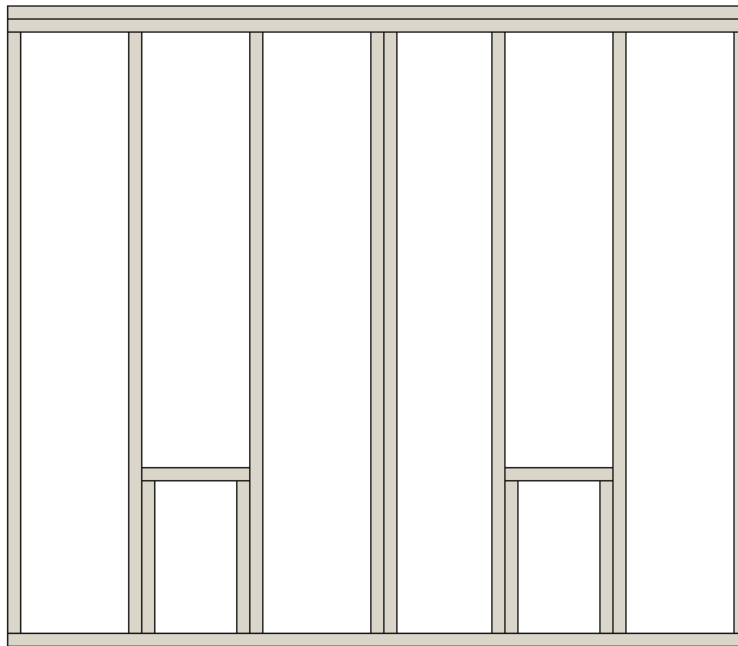
Figure 2. Typical Construction of Two Adjacent Test Wall Specimens
