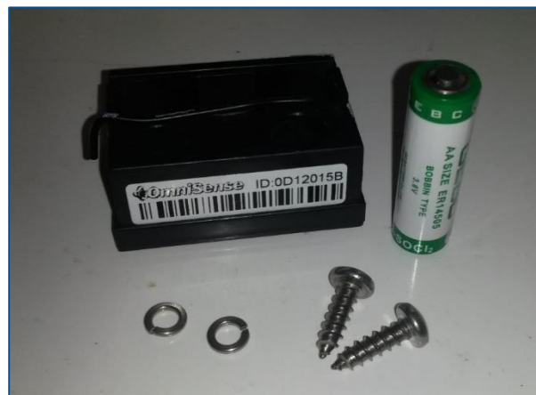
Figure 6. Wireless Temperature, Humidity and Wood Moisture Sensor
