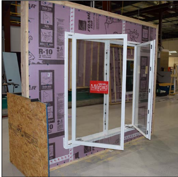
Figure 35. Muller Casement Window on 2 in. of 15-psi XPS
