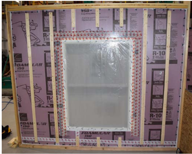
Figure 33. 2 in. of 15-psi XPS - Single DH
