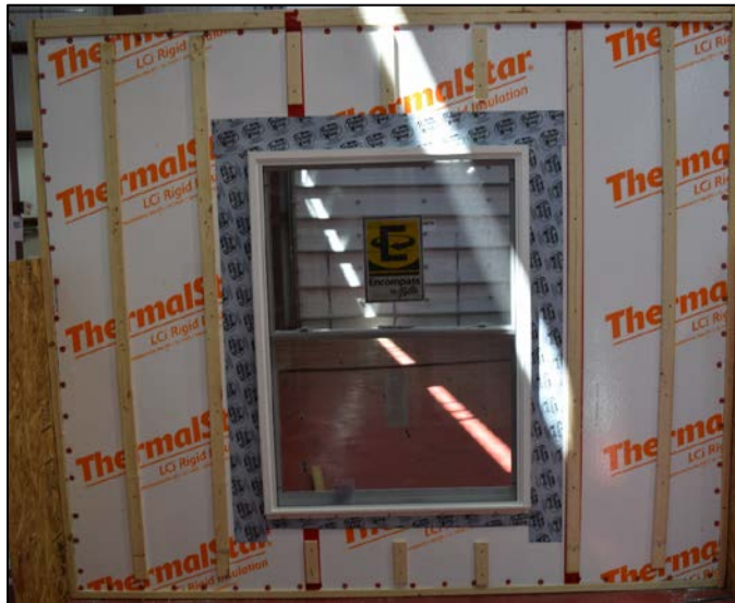
Figure 29. 1 in. of 15-psi EPS - Single DH
