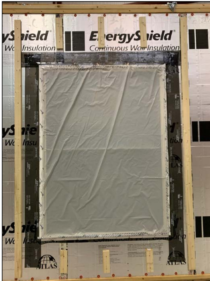
Figure 30. 1 in. of 16-psi PIR - Single DH
