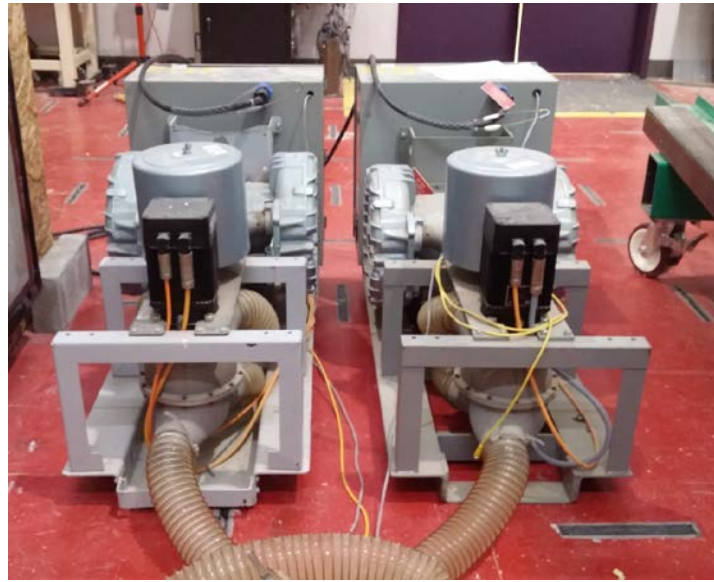
Figure 10. Pressure Load Actuators
