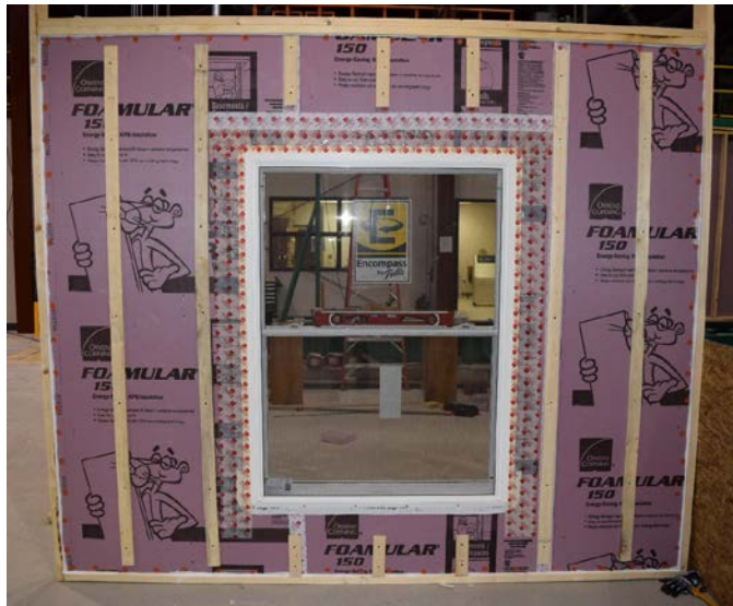
Figure 26. 1 in. of 15-psi XPS and OSB - Single DH
