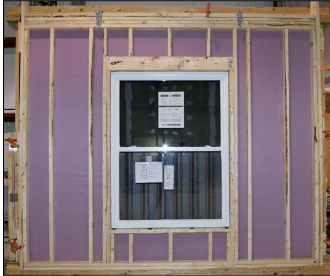
Figure 28. 1 in. of 25-psi XPS and No OSB - Single DH
