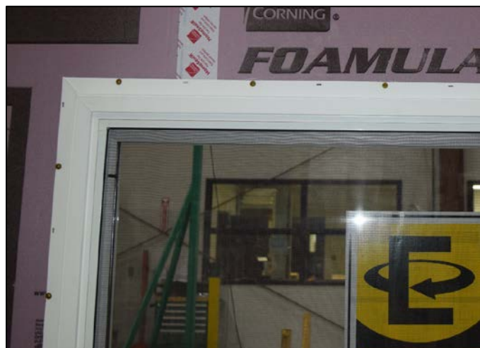
Figure 34. Cabinet Screw Installed on 2 in. of 15-psi XPS - Single DH
