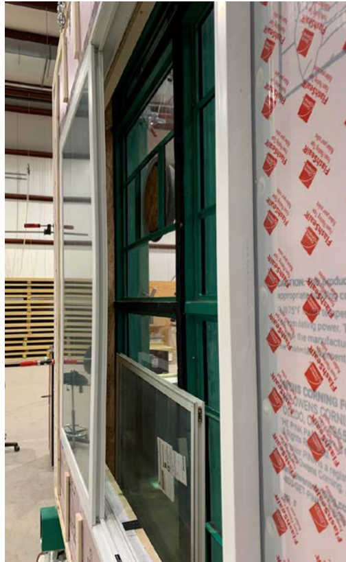
Figure 21. Window Being Pulled Off Its Sash
