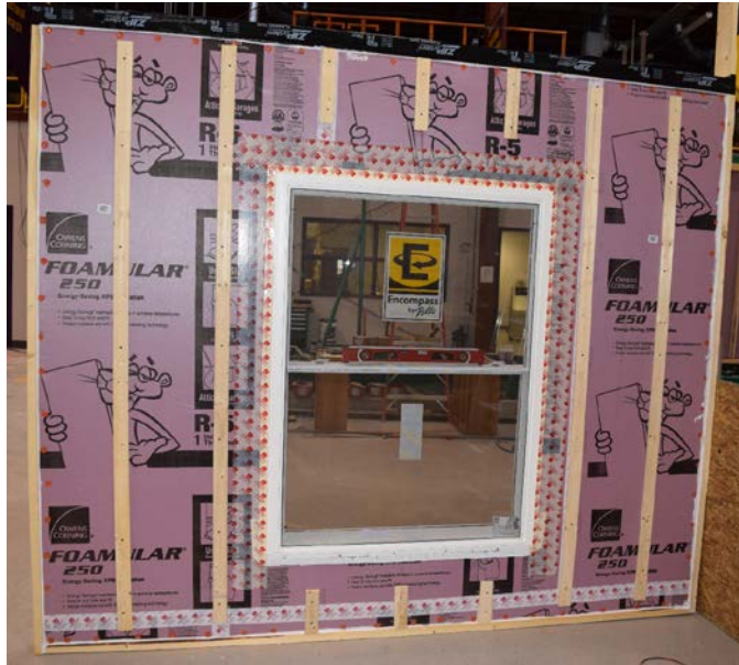
Figure 27. 1 in. of 25-psi XPS and OSB - Single DH
