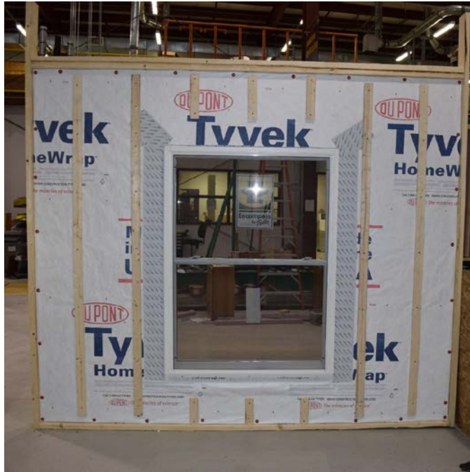
Figure 22. Housewrap and OSB – Single DH
