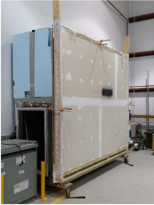
Figure 5. Wind-Blown Rain/Air Infiltration Test Chamber for Air Leakage
