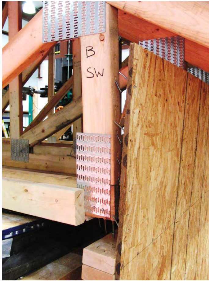
Figure 12 – Fastener yield and pull-through failure mode of Test B
