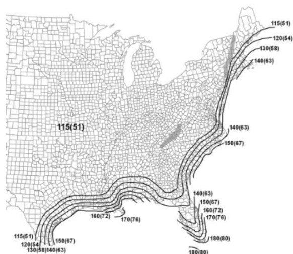
FIGURE 2. Wind Regions. Source: Figure R301.2(5)A Excerpted from the 2018 International Residential Code; Copyright 2017; Washington, D.C.: International Code Council. Reproduced with permission. All rights reserved. www.ICCSAFE.org
