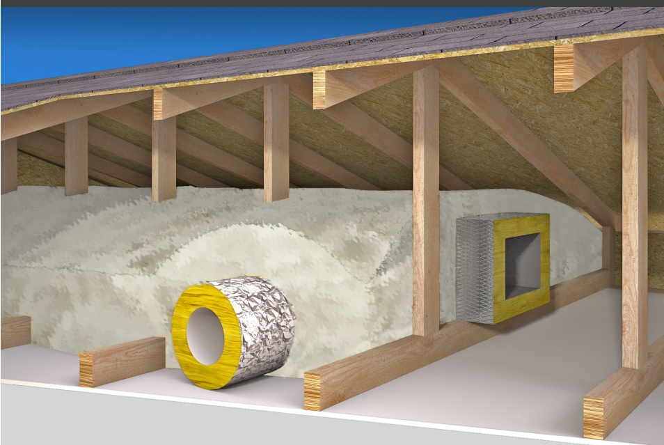
Figure 1. Buried Ducts: Insulated HVAC Ducts Buried within Fiberglass Ceiling Insulation.
