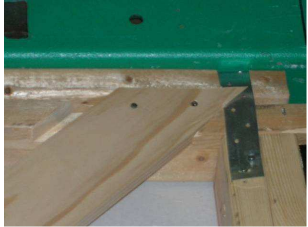
Figure 18 – Configuration 12 (Shear plug failure at compression brace)
