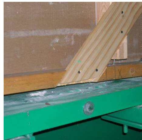
Figure 16 – Configuration 8 (Tension brace connection performance)
