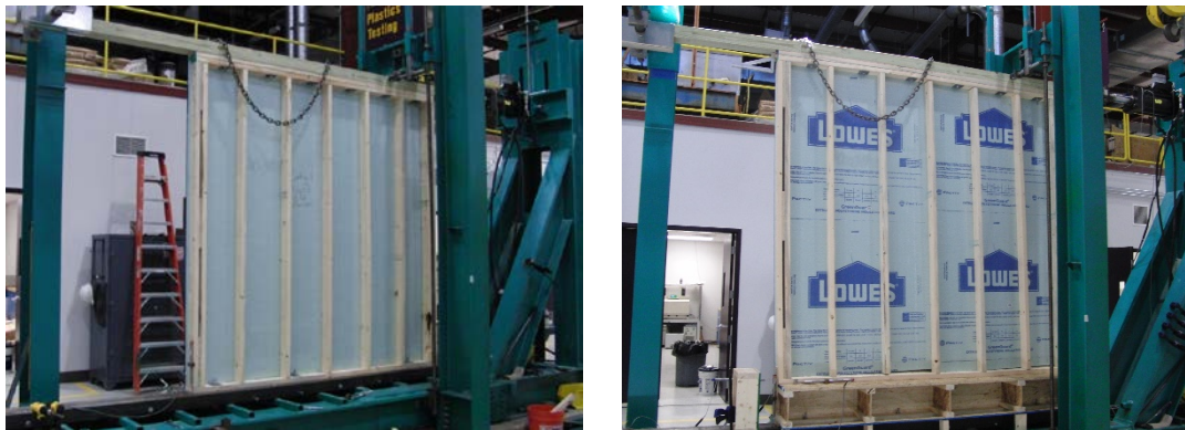
Figure 6. Specimen in test setup with and without floor platform
