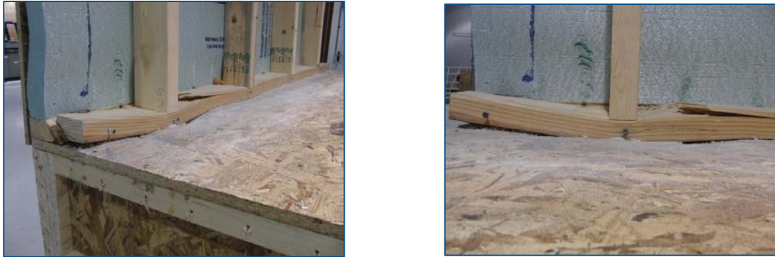
Figure 10. Primary failure mode of compression test
