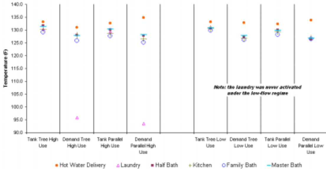
Figure 18. Experimental maximum delivery temperatures for each outlet
