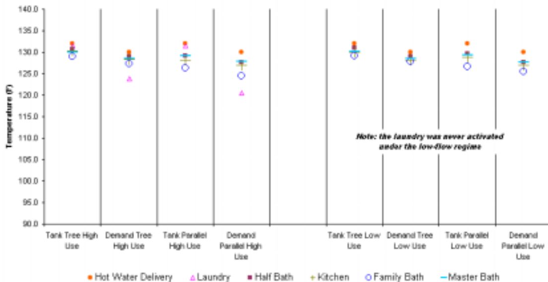
Figure 19. Simulated maximum hot water delivery temperatures
