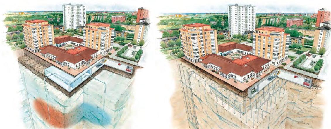
Figure 2: Aquifer Thermal Energy Storage (ATES) (left) and Borehole Thermal Energy Storage (BTES) (right). Illustration: Geotec.
