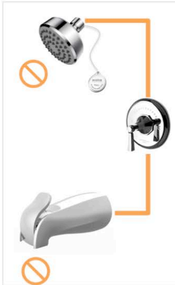
5. Specialized showerhead trickles by default so hot water is not flowing until user is ready to shower.
