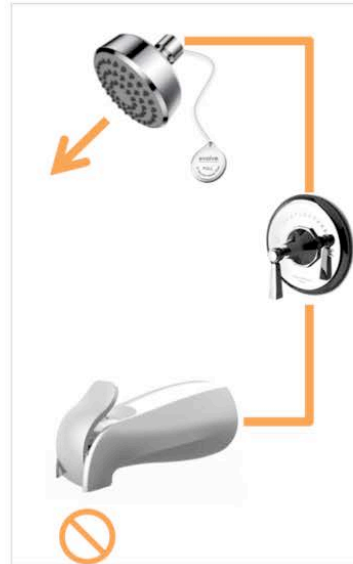
6. User pulls cord to activate specialized showerhead's normal flow and begins showering.
