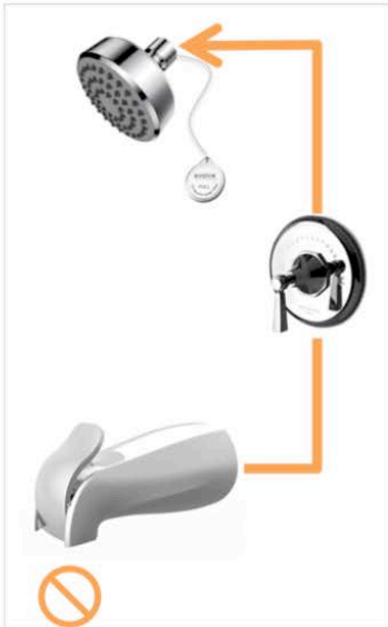
4. Hot water is automatically diverted to specialized showerhead (integrated normally closed valve).
