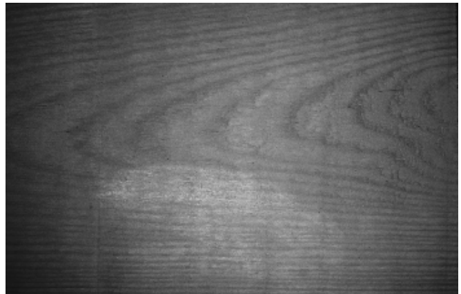
Figure 11—Shiny area on wood surface caused by excessive buildup of binder from waterborne WRP.
