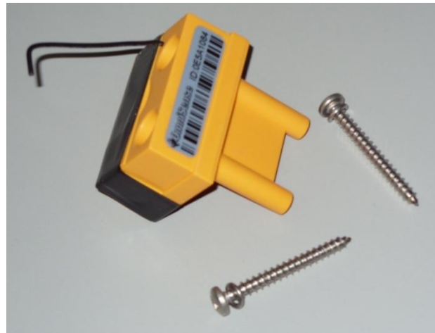
Figure 6. Wireless Temperature, Humidity & Wood Moisture Sensor
