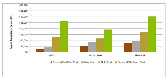
Figure 6. Cost of Rating System Compliance – Denver, CO, Climate Zone 5, 2009 IECC Compliant
