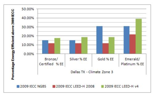
Figure 11. Simulated Energy Efficiency at Rated Level for Each System
