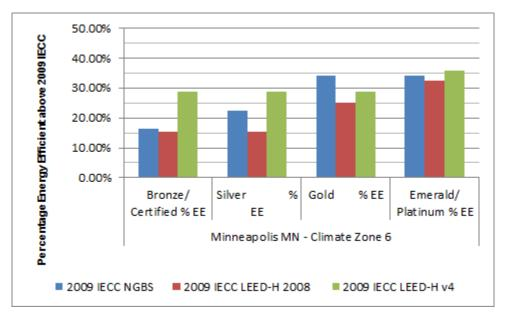
Figure 13. Simulated Energy Efficiency at Rated Level for Each System
