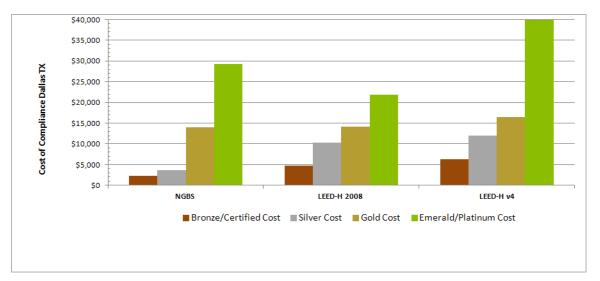
Figure 5. Cost of Rating System Compliance – Dallas, TX, Climate Zone 3, 2009 IECC Compliant
