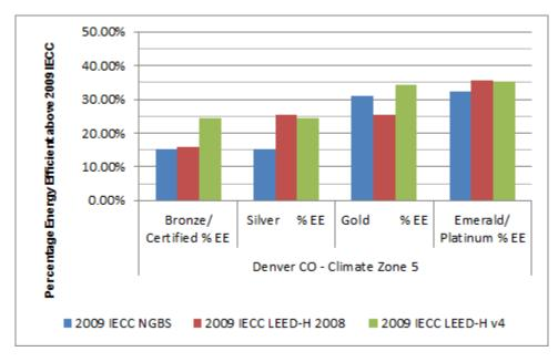
Figure 12. Simulated Energy Efficiency at Rated Level for Each System
