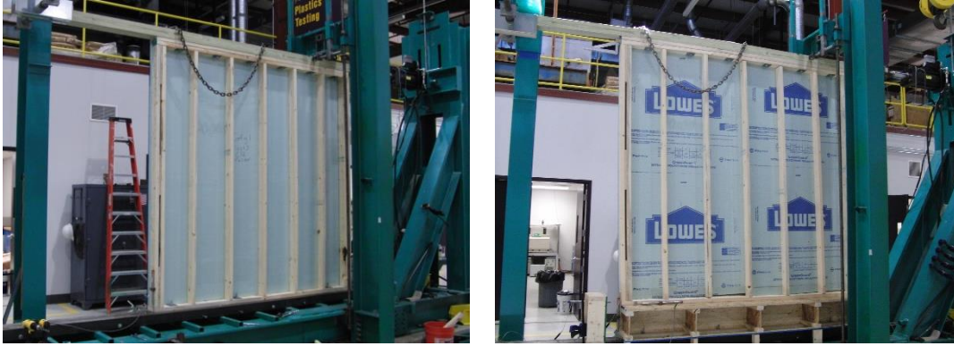
Figure 7 Specimen in Test Setup with and without floor platform
