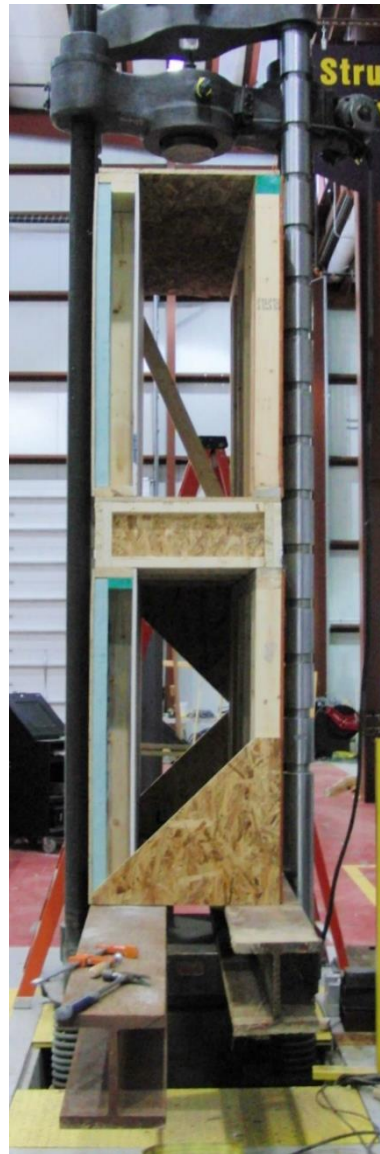
Figure 8. Configuration 3 Test Setup with Temporary Bracing
