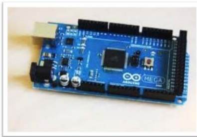
Figure 8 Arduino Mega 2560 that replaced the PLC.
