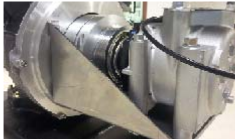
Figure 11 Compressor directly couple to engine flywheel.
