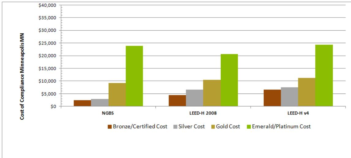
Figure 16. Cost of Rating System Compliance – Minneapolis MN, Climate Zone 6, 2012 IECC Compliant
