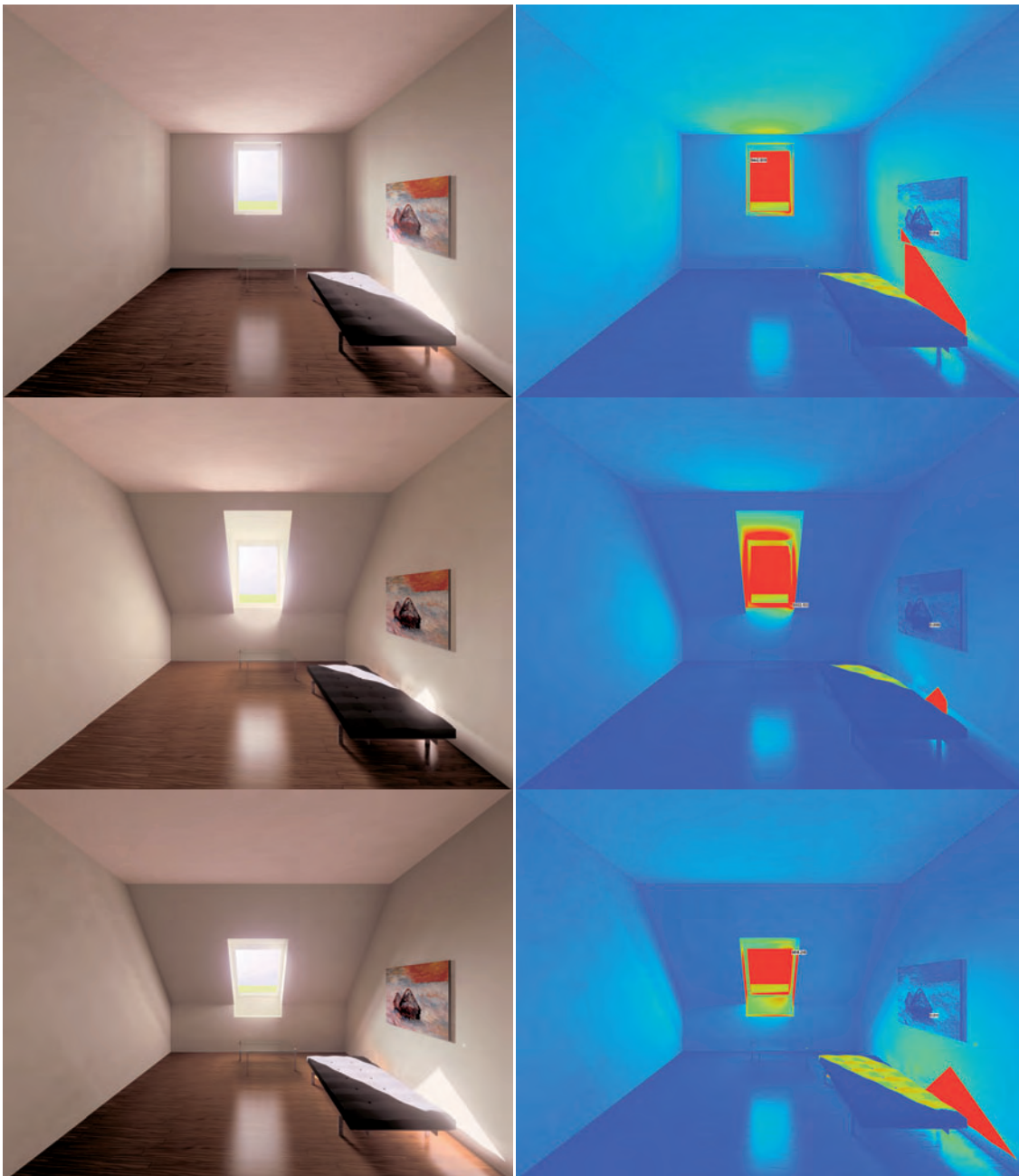
Figure 94. Radiance pcond and false colour renderings for the three rooms with furniture.
