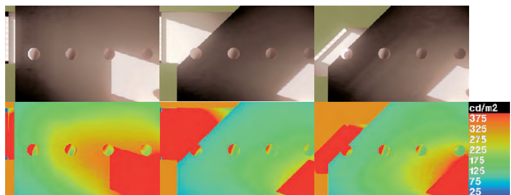
Figure 74. West facing in March at 16:00: The sunlight hits the back wall, and therefore the diffuse inter-reflected light dominates in the depth of the rooms.
