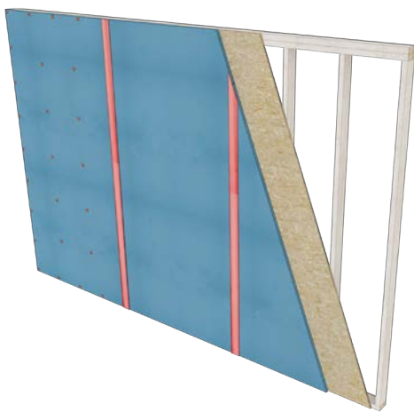
Figure 21. Example Exterior Air Barrier (Taped Foam Sheathing)
