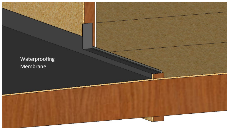
Figure 6. Install Waterproofing Membrane
