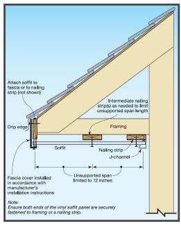
loads and, for vented soffits, are resistant to water intrusion. As a best practice, aluminum soffit panels should meet the same requirements. The IRC also has minimum requirements for wood structural panel soffits.
