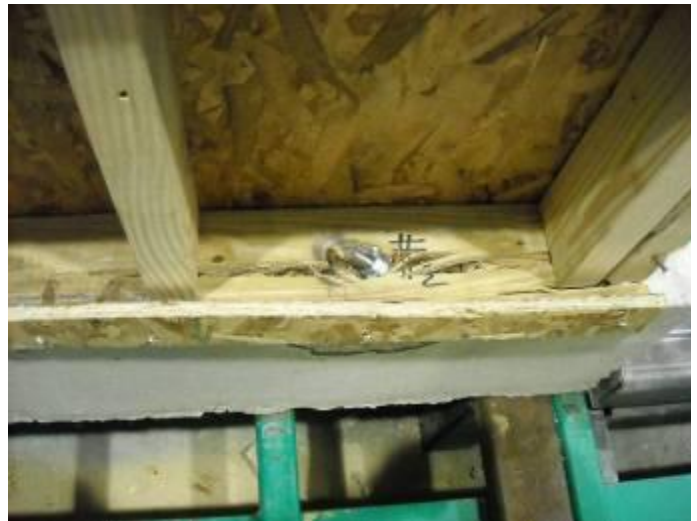
Figure 24 – Plate degradation in full-scale shear wall test with round cut washers
