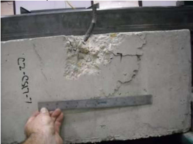
Figure 14 – Final large spall in monotonic test of 2x4 plate with plate washer
