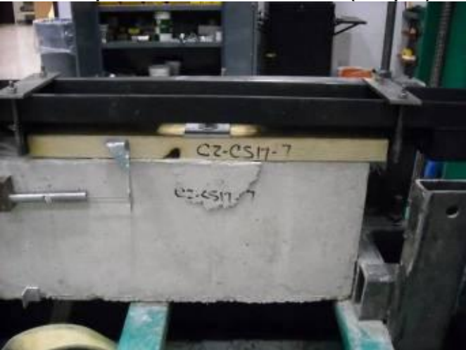
Figure 13 – Initial spall in monotonic test of 2x4 plate with plate washer
