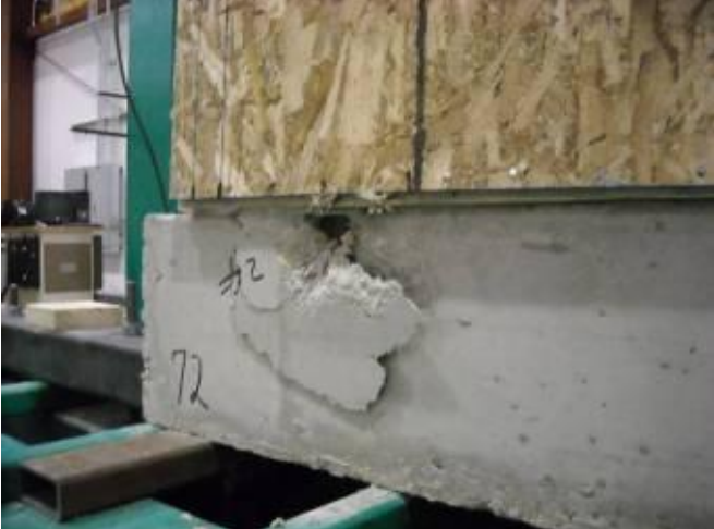
Figure 25 – Large spall in third monotonic full-scale shear wall test
