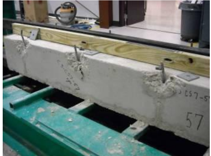
Figure 21 – Tensile failure of bolts in Configuration 3 test
