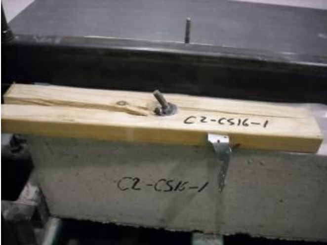
Figure 11 – Plate splitting failure in monotonic test of 2x4 plate with round cut washer (no spall)
