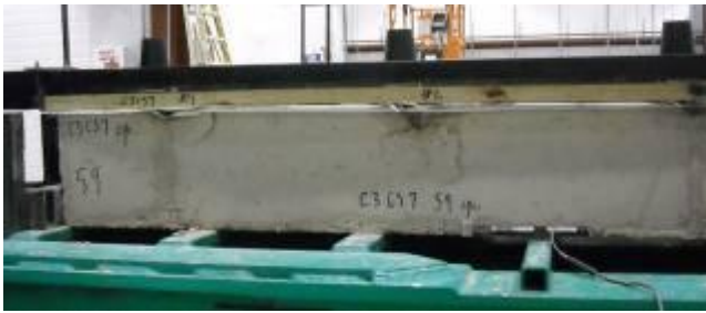
Figure 20 – Large spall at center bolt in Configuration 3 test
