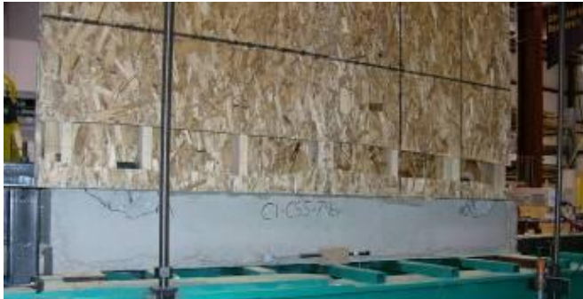
Figure 26 – Failure of full-scale shear wall specimen during cyclic testing (sheathing removed post-test to allow for inspection)
