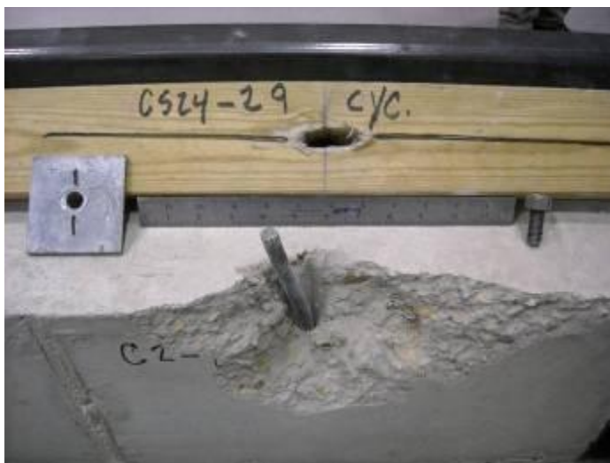
Figure 18 – Tensile failure of bolt in Configuration 2 test
