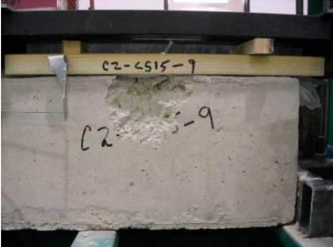
Figure 12 – Minor spalling in monotonic test of 2x4 plate with round cut washer
