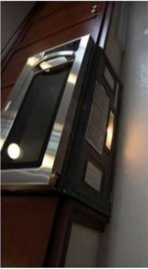
Figure 17: The dimensions and irregular surface of this typical microwave-integrated range hood in FH2 makes inlet flow measurements difficult
