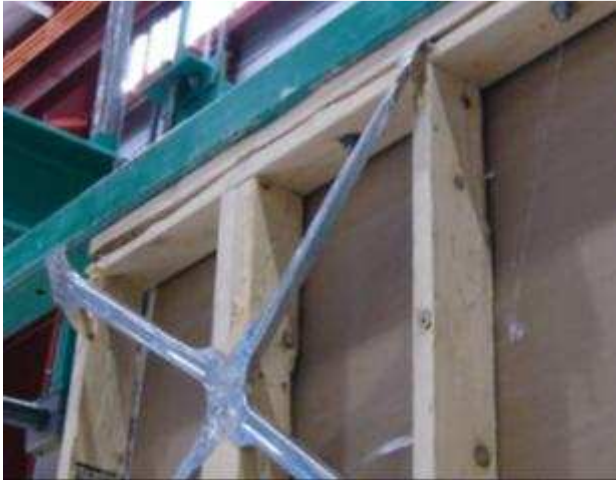
Figure 21 – Withdrawal failure of web members (Specimen K)
