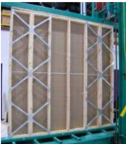
Figure 15 – Specimen L wall construction
