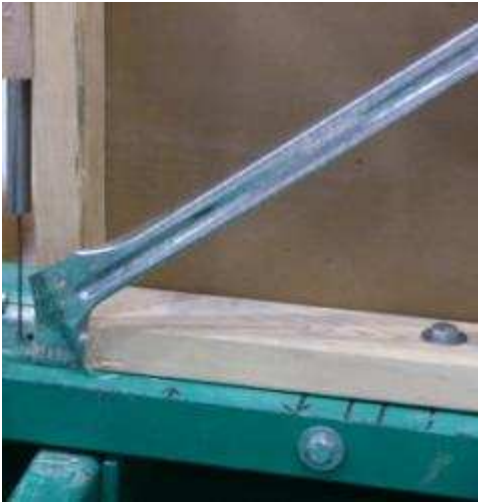
Figure 19 – Combined buckling and withdraw failure at trailing edge of wall (Specimen K)
