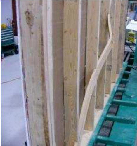
Figure 7 – Buckling failure of wood brace (Specimen D)
