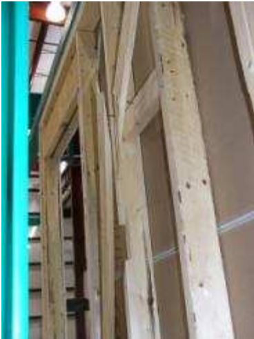
Figure 10 – Buckling failure of wood brace (Specimen G)
