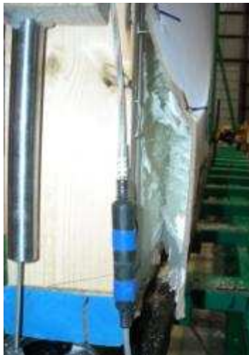
Figure 35 – Separation of SPF from sheathing (Specimen S)
