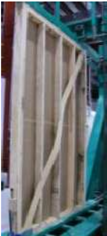
Figure 8 – Out-of-plane bending of wood brace (Specimen E)
