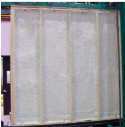
Figure 31 – Flash & batt application of SPF (Specimen R)
