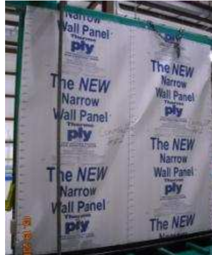
Figure 34 – Buckling failure of sheathing (Specimen S)
