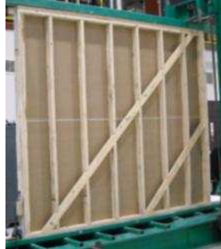
Figure 14 – Specimen I wall construction
