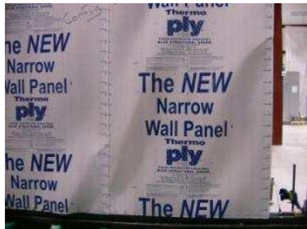
Figure 32 – Buckling failure of sheathing (Specimen R)
