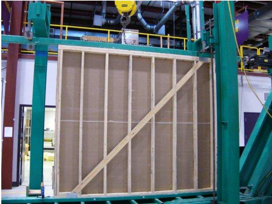
Figure 2 – Shear wall test specimen (Specimen D)
