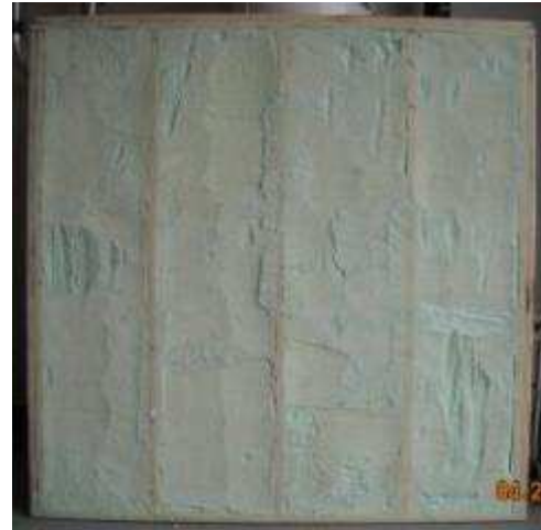
Figure 28 – Full cavity SPF application (Specimen Q)
