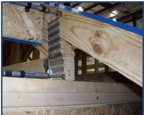
Figure 14 – Truss member displacement and metal connector plate deformation at heel joint (Specimen A)
