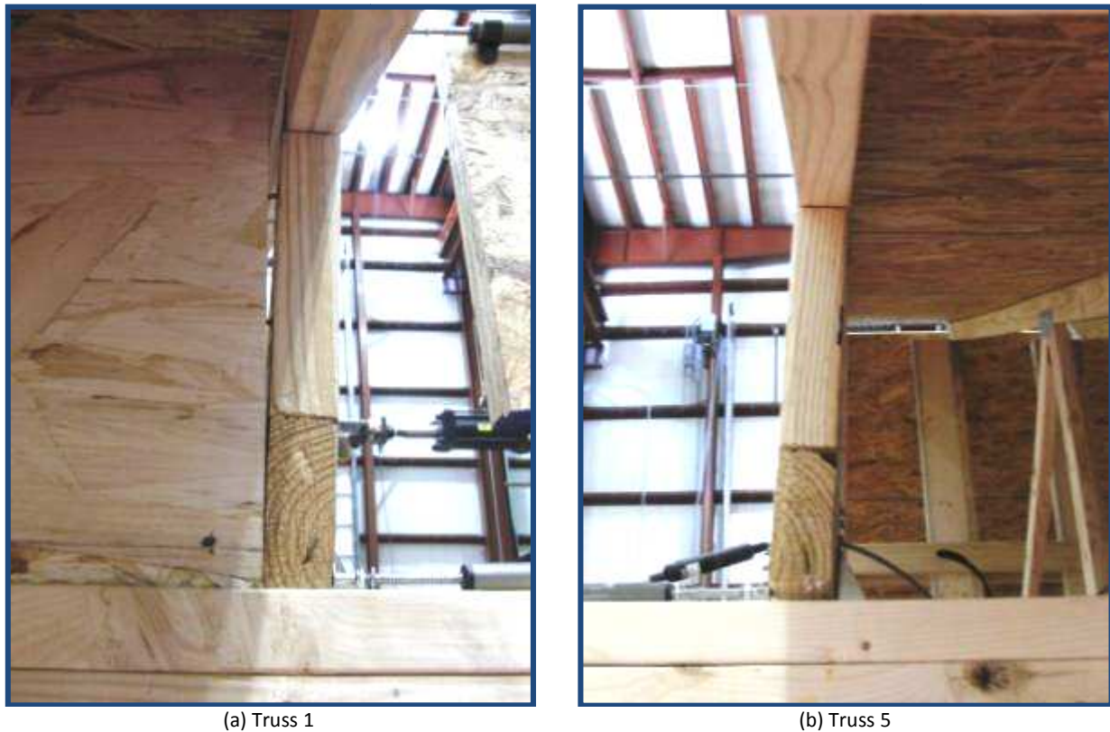
(a) Truss 1 (b) Truss 5 Figure 19 – Comparison of truss heel rotation (Specimen F)
