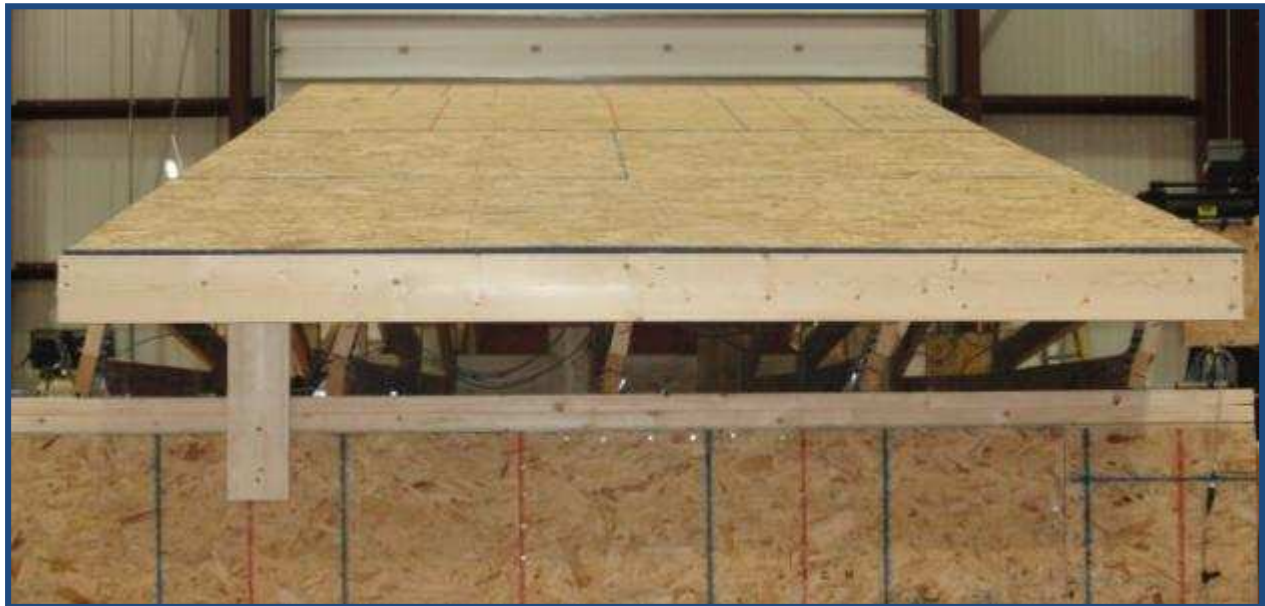
Figure 16 – Specimen C heel rotation at failure
