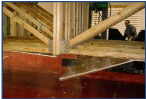
Figure 12 – Complete failure of gypsum fasteners (Specimen A)
