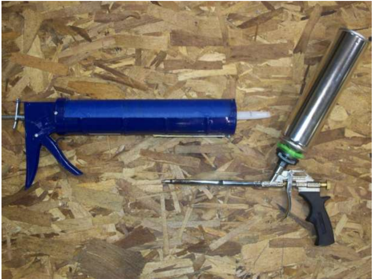
Figure 2: Cartridge subfloor adhesive and applicator (Left) and DAP adhesive and applicator (right)
