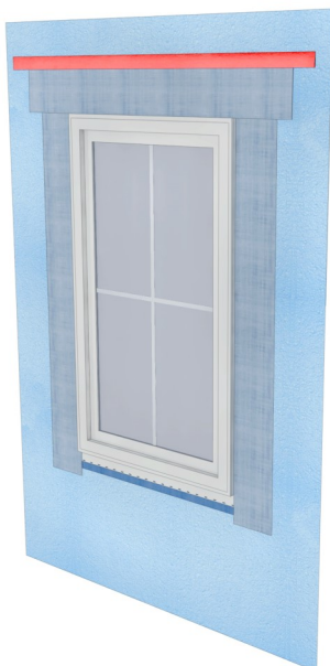
Figure 4. Example flashing details for a flanged window installed over rigid foam insulation sheathing installed as the WRB.
